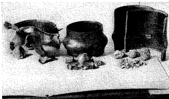
FIG. 8. Photograph of solid metal rotors and vacuum chambers after explosion by centrifugal force.
